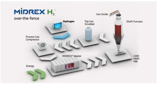
Figure 5a. MIDREX H<sub>2</sub> with hydrogen supplied over-the-fence
