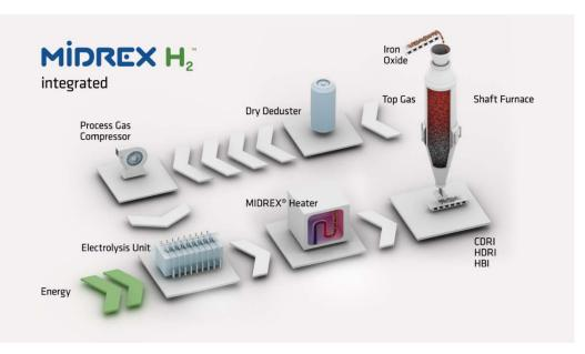
Figure 5b. MIDREX H<sub>2</sub> with integrated hydrogen generation
