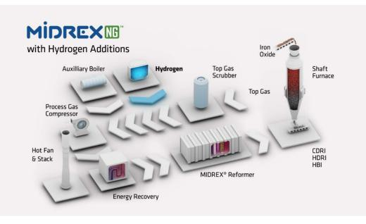
Figure 4. MIDREX NG Process with hydrogen addition: more than 30% natural gas displacement
